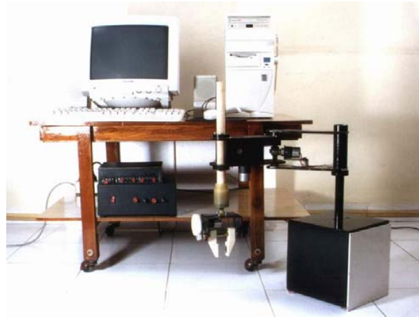
Fig. 3 The computer controlled SCARA robot
