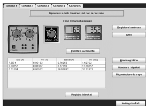
Fig. 4 One page of FIL belonging to the virtual laboratory on the Hall effect
