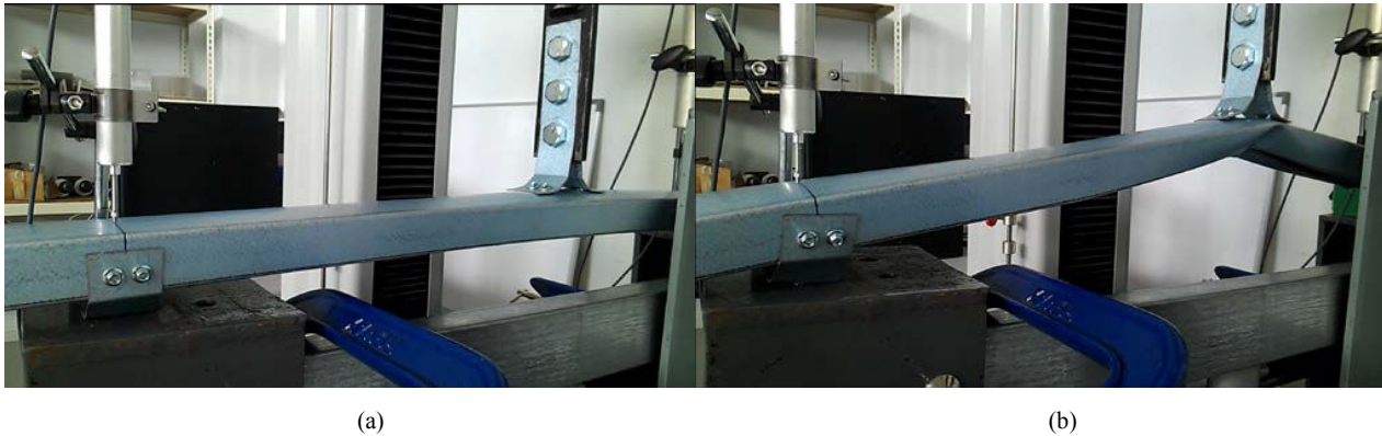
Fig. 7 (a) First observed failure mode and (b) second observed failure mode in the first parametric study
