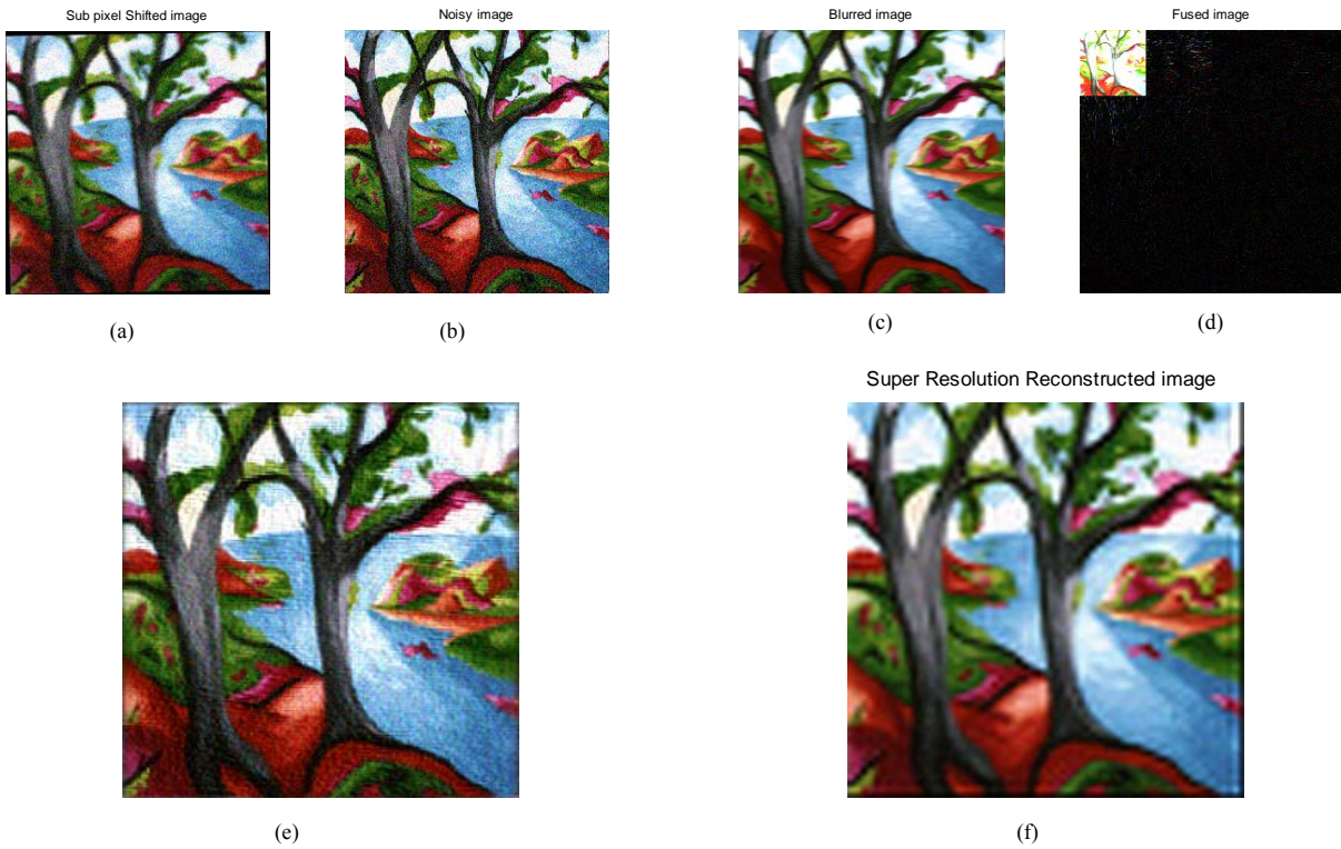
Fig .3 (a) Sub pixel shifted low resolution image (b) Noisy low resolution image (c) Blurred low resolution images with a BSNR of 40 db (d) Wavelet decomposed fused image (e) Super resolution blind reconstruction using zonal filter and blind deconvolution (f) Super resolution blind reconstruction using wavelet based fusion with an ISNR of 5.56 db at 0.56 bit rate
