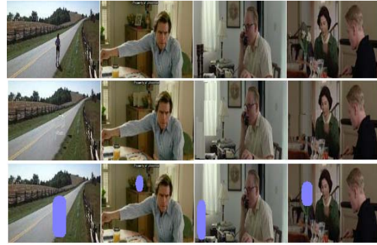
Fig. 5 Row 1: Screenshots from Internet streamed video sequences; Row 2: Copy-move tamper emulation for the scene; Row 3: Detection of tampered regions in the scene
