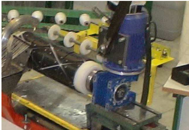
Fig. 1 Fabrication Process with filament winding method
