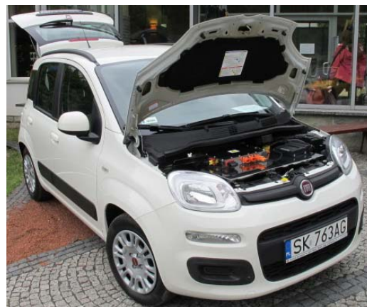
Fig. 2 Fiat Panda with Komel's traction motor – research and development project no. NR01-0084-10
