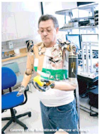
Fig. 7 Eight Degrees of Freedom Bionic Arm of the RIC controlled by “thought” (see text).
