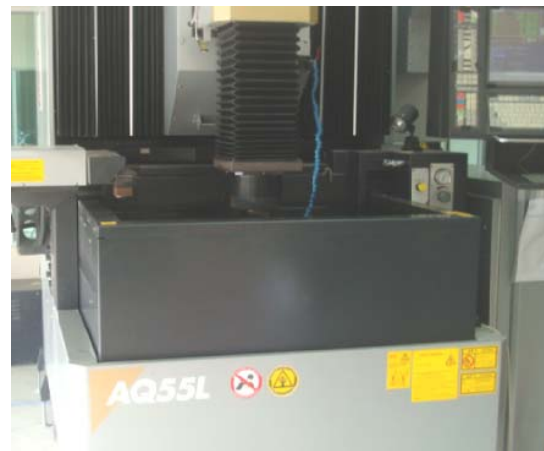
(b) EDM tank with electrode and workpiece.
