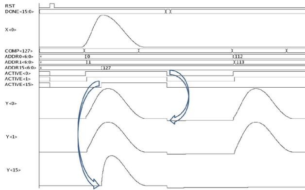
Fig. 2 The mixed-signal switching time diagram
