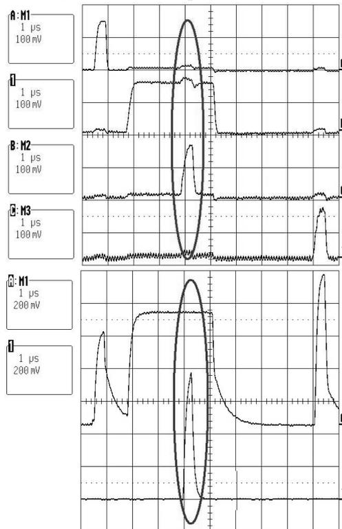
Fig. 7 The switching of the 4 read-out channels (top) to 2 processing ones (bottom)
