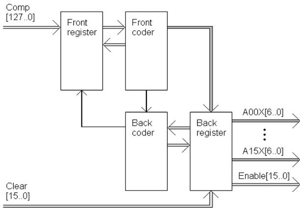
Fig. 5 The arbitration logic
