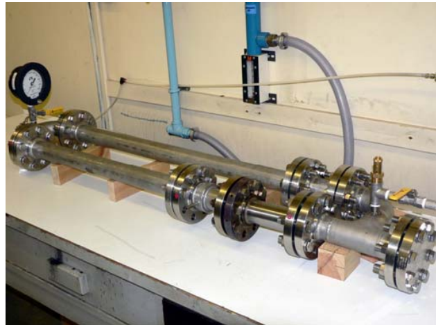
Fig. 2 Looped tube travelling-wave thermoacoustic engine
