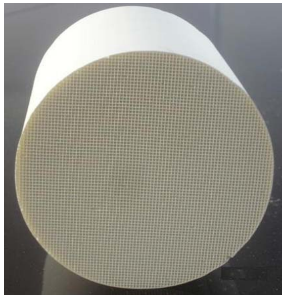
Fig. 3 The ceramic regenerator
