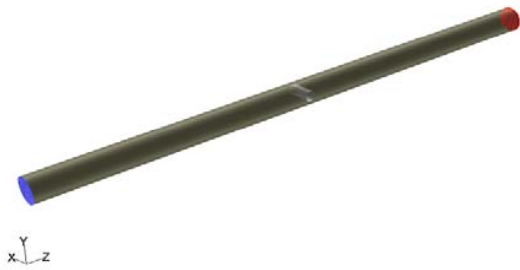
Fig. 13: Geometry of the flow inside the tube and excitation using 4mm diameter cylindrical block
