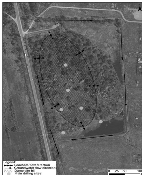
Fig. 2 Kleisti Dump Site (Nr. 1 in Fig. 1) Location of drilling sites, leachate and groundwater flow directions
