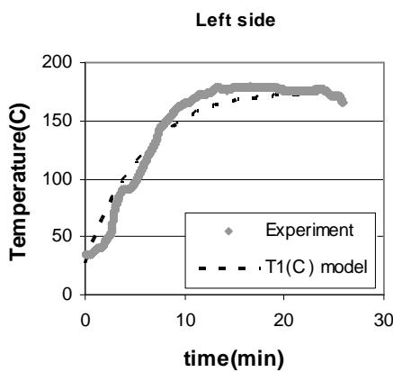
Fig.6. Left side, car body temperature vs time
