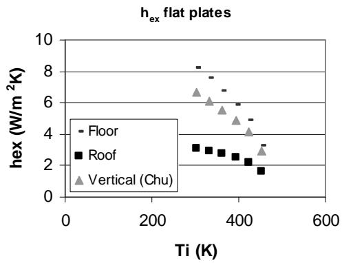
Fig.3. Flat plate  $h_{B_{exB}}$  vs car body temperature
