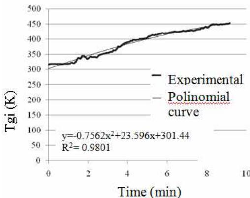
Fig.4. Internal gas temperature ( $T_{gi}$ ) vs time
