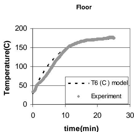
Fig.11. Floor, car body temperature vs time
