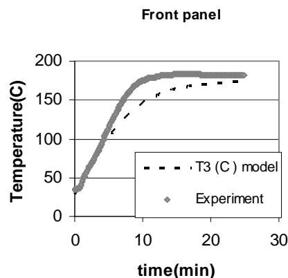
Fig.8. Front side, car body temperature vs time
