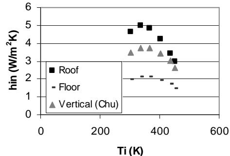
Fig. 5. Flat plate  $h_{in}$  vs car body temperature
