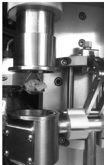
Fig. 2 Placing of the sample into the DVS device
