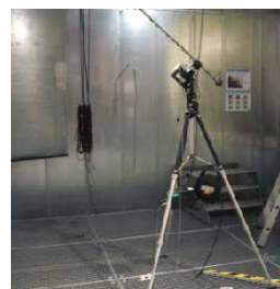
Fig. 4 Rotating "Galgen" for determining average sound pressure level
