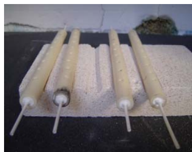
Fig. 5 Photographs of fibres mounted into their mechanical dense alumina support with a new layer of enamel tube. Step before sealing and enamelling
