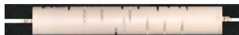
Fig. 4 (b) Schematic mounting of the fibre before sealing enamel at 600°C in a dense alumina tube with holes
