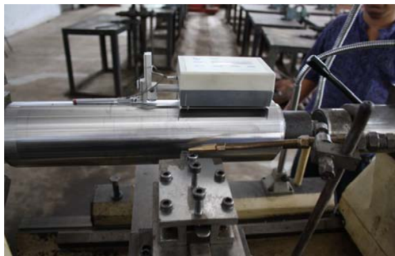
Fig.2 Photographic view of surface roughness measuring technique
