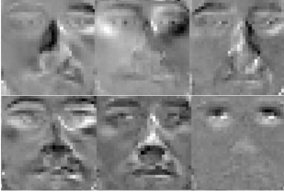
Fig. 5 Example of the first eigenobjects (eigenfaces)
