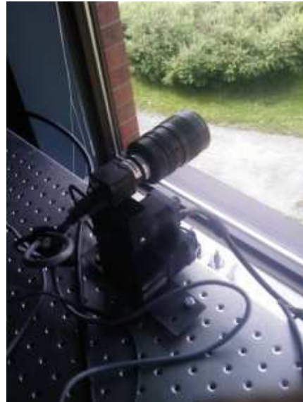
Fig. 6 Pan and Tilt unit PTU-D46-17with a 1024x768 camera
