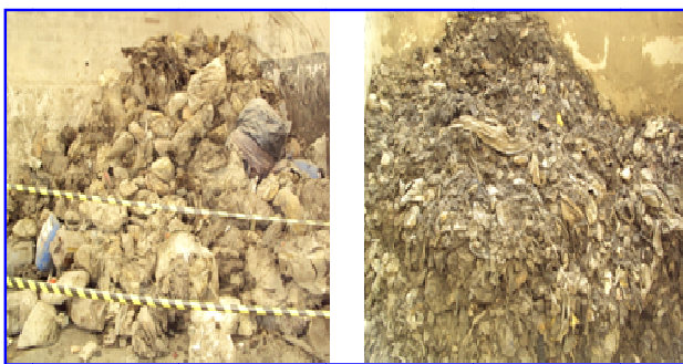
Fig. 6 MR 200 rejecting material which consists holds granulometry larger than 200 mm.
