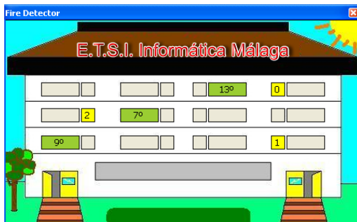
Fig. 7. Fire Detector Screen.
