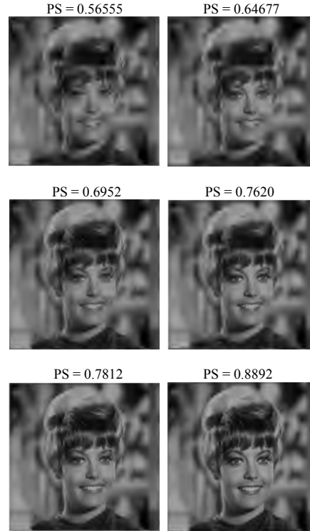
Fig. 10 “Zelda” image compression results. The images of the left column that follow are for SPIHT ONLY coded images. The images of the right column that follow are for the visually optimized SPIHT POEFIC coded images. The bit rates from top to bottom are 0.03125 bpp, 0.0625 bpp and 0.25 bpp respectively, at observation distance of V = 4
