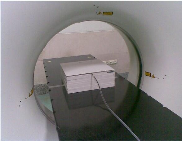
Fig. 1 phantom placed in CT scan device
