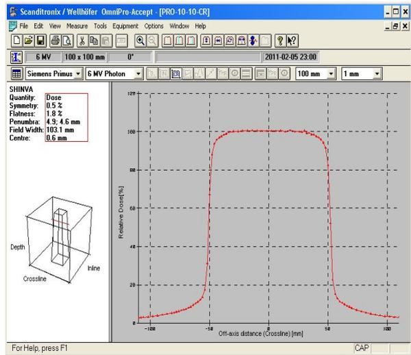
Fig. 3 Standard Field (10\*10) Measurement With semiconductor
