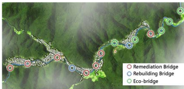
Fig. 11 Suggestion on walking bridge reconstruction
