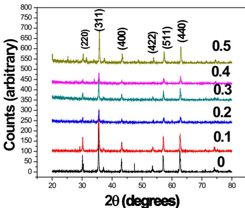
Fig. 1 XRD patterns for  $\text{CoFe}_{2-x}\text{Cr}_x\text{O}_4$  where  $x=0.0, 0.1, 0.2, 0.3, 0.4, 0.5$ (sintered)
