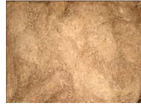
Fig. 2 Oil palm fibres (OF)
