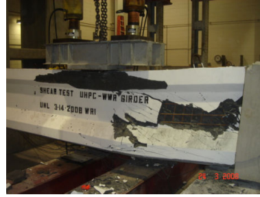
Fig. 8 Girder test (limit state)
