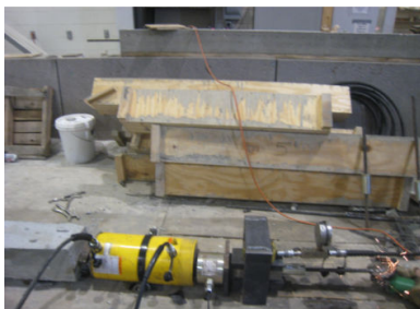
Fig. 4 Pullout test setup and strand gripping
