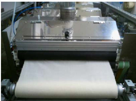
Fig. 1 Innovative Veneto Nanotech machine Nanofabia for in-line treatment of fibrous and web materials
