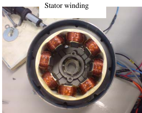
Fig. 1 4 phases SRG stator poles and winding
