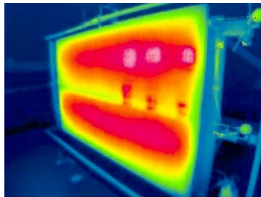
Fig. 7 Illustration of thermo-camera monitoring: warming
