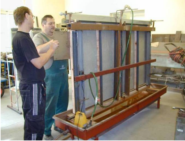
Fig. 14 Installation of test specimen and test equipment for warming and sprinkling fiber-cement slab
