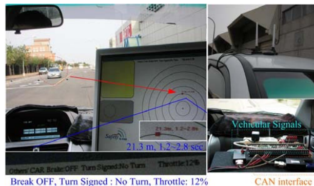
Fig. 16: Remote warning test in short range.
