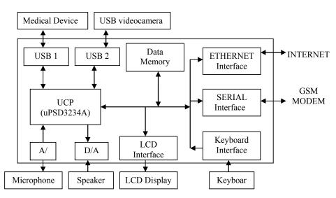
Fig. 2 The biosignal / ECG telemonitoring unit of our project
