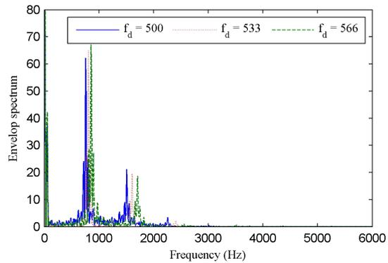
Fig. 4b Envelope spectrum of the vibration signal
