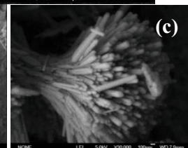
Fig. 6 SEM of the typical product obtained from steelmaking slag with employing filtrate from former enhanced carbonation step as leaching medium: (a) an overview of the formed particles; (b) and (c) magnified views of the product.
