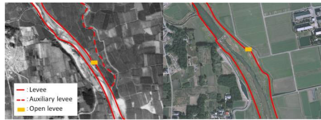
Fig. 4 Plan views of the Jobaru River before (left) and after (right) construction of disaster subsidy projects
