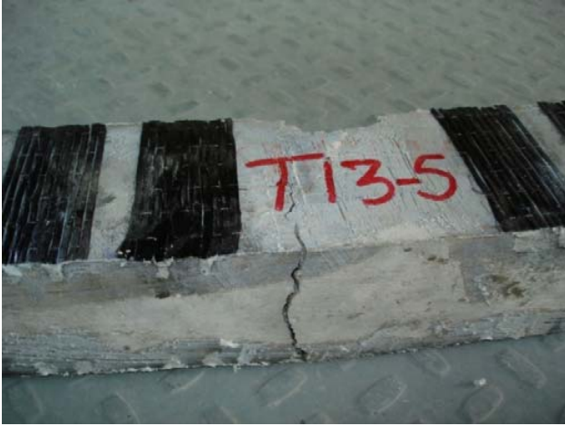
Fig. 8 Specimen prepared with grooving method
