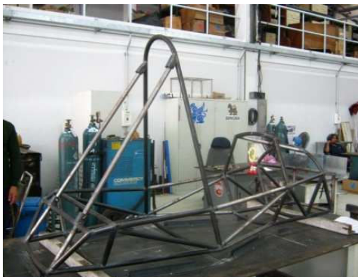
Fig. 3 The 2011 frame for 2011-2012 Auto Challenge student formula
