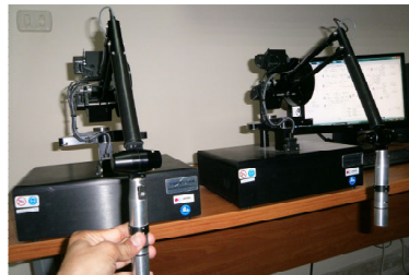
Fig. 7 bilateral teleoperation system using two Phantoms
