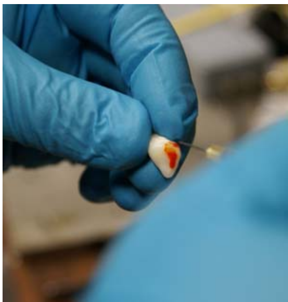
Fig. 8. Applying the fluorescence agent on the tooth resin interface for sample 79.
