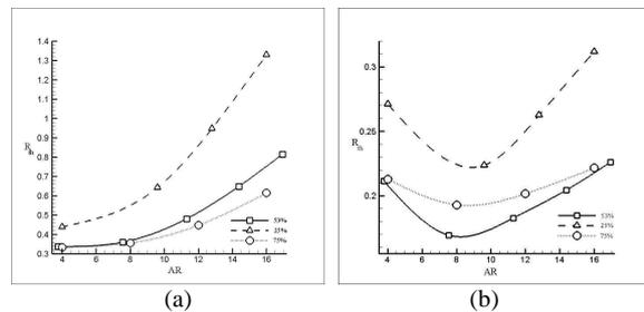
Fig. 4 Effect of porosity applying pressure (a) 490Pa; and (b) 2940Pa
