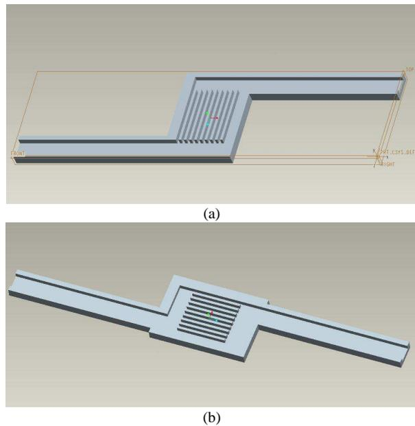
Fig. 5 Entrance arrangement configuration: (a) Type-2;(b)Type-3
