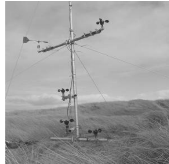
Fig. 3 Mast cup anemometers were installed at 0.2 m, 0.5 m, 1 m, 2 m and 5 m heights
