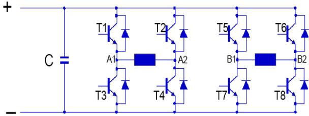
Fig. 11. Inverter considered for BLDC with Two-Phase Winding
