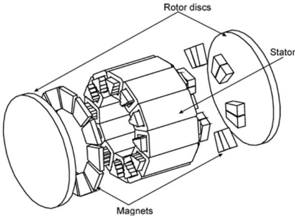
Fig 1 Double-sided AFPM motor with two external rotors
