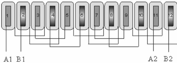
Fig. 2 Windings of the stator is connected in Two - phase
