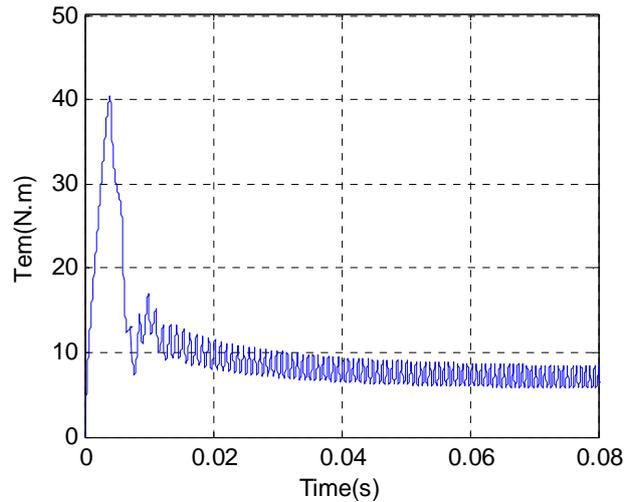
Fig. 9 Waveform of electromagnetic torque ( $T_{em}$ )
