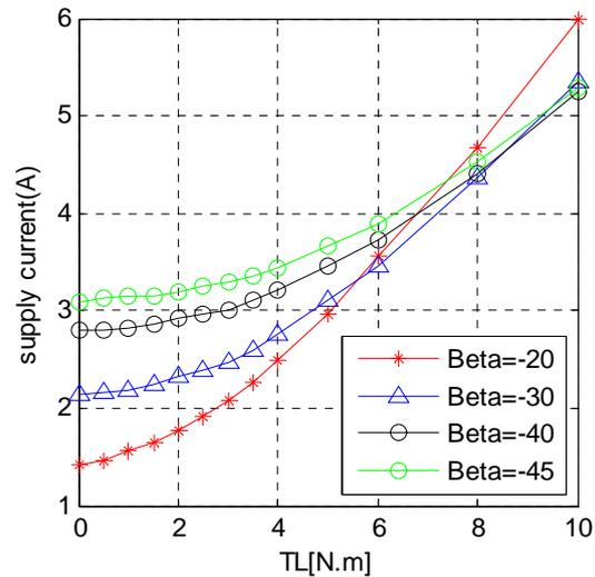
Fig. 14 Input current (Is) vs. load torque(TL)
