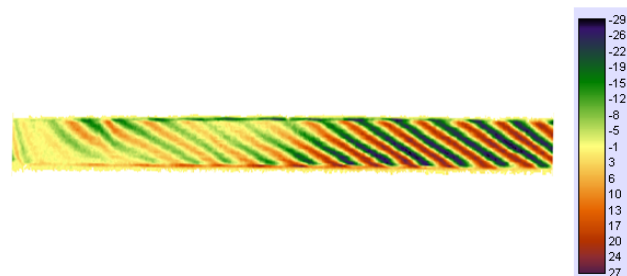
Fig. 2 Isodeformation map associated to the loading specimen 1 loaded with 50 N
