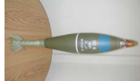
Fig. 2 The non-rolling finned 120 mm HE mortar projectile
