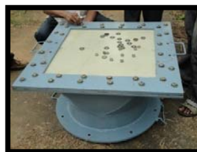
Fig. 1 FRP laminate fixing to the underwater shock test setup fixture
