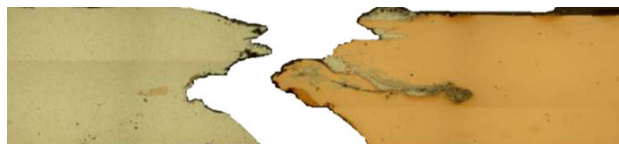
Fig. 3 (b) Fractured surface of weld produced at 1200 rpm and 300 mm/min with the 25 mm shoulder diameter tool
