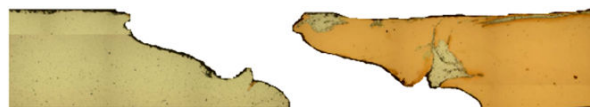
Fig. 3 (a) Fractured surface of weld produced at 950 rpm and 300 mm/min with the 25 mm shoulder diameter tool
