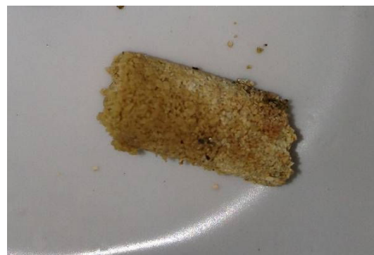
Fig. 9 Sintering of composite catalyst bed after test
