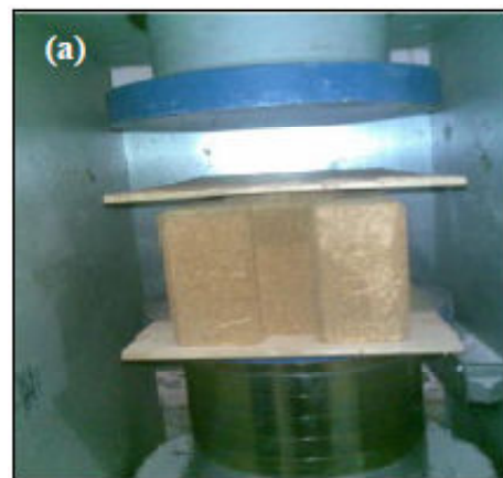
Fig. 3 Test set-up for compression test
