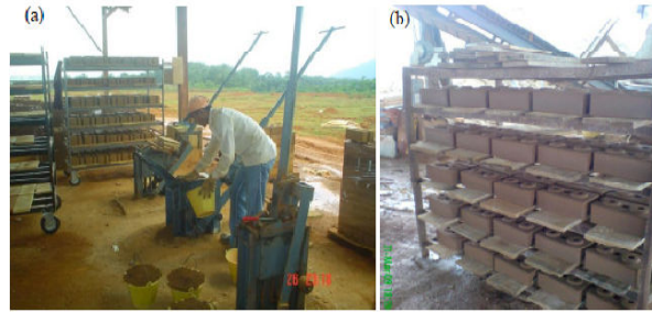
Fig. 2 Interlocking brick; (a) mould for pressing and (b) curing process
