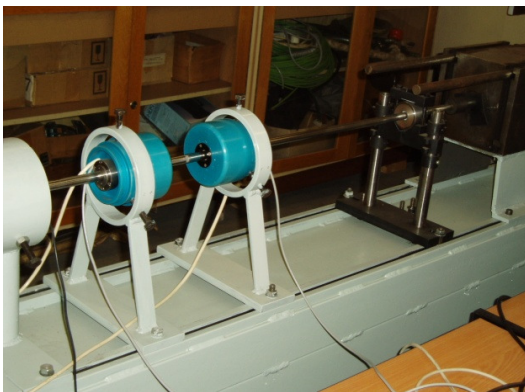
Fig. 2 The Split Hopkinson Pressure Bar
