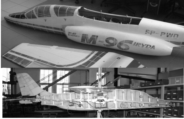
Fig. 2 airplane model for flutter testing (from top): external geometry of the airframe, the internal structure of the airframe
